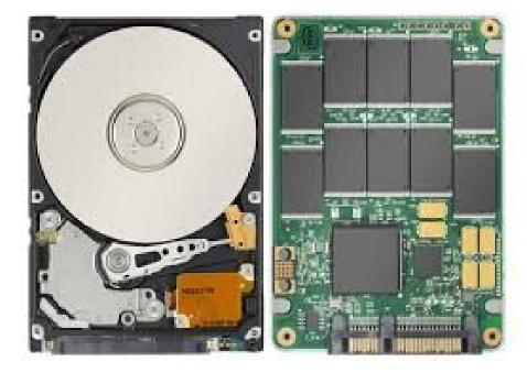
The storage disk of a computer is the non-volatile storage device. This is where all the files and programmes you have saved on your computer reside. Unlike the RAM which is volatile, the storage disk still retains data even when there is no power running through the computer (there is the reason for its non-volatile reference). The capacity of the storage disk is usually higher than that of the RAM since it is the "storage bank" for the component.
